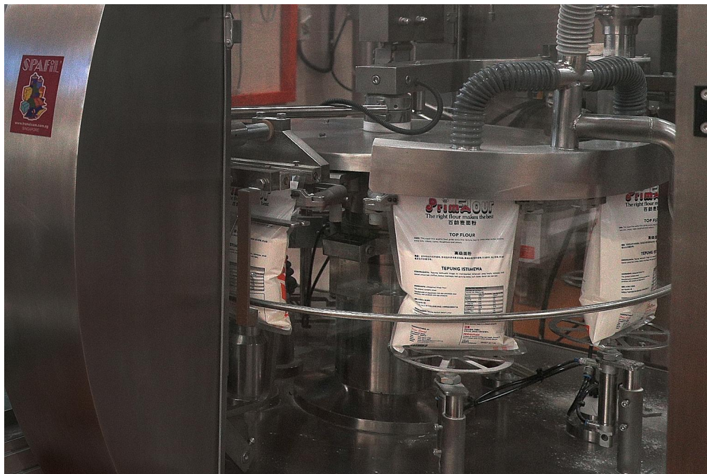
Prima's new machine was sourced and installed in nine days, with teams working two weekends and public holidays to get it up and running. The new line increased its packing capacity for household packs by 75 per cent. ST PHOTO: JASON QUAH
